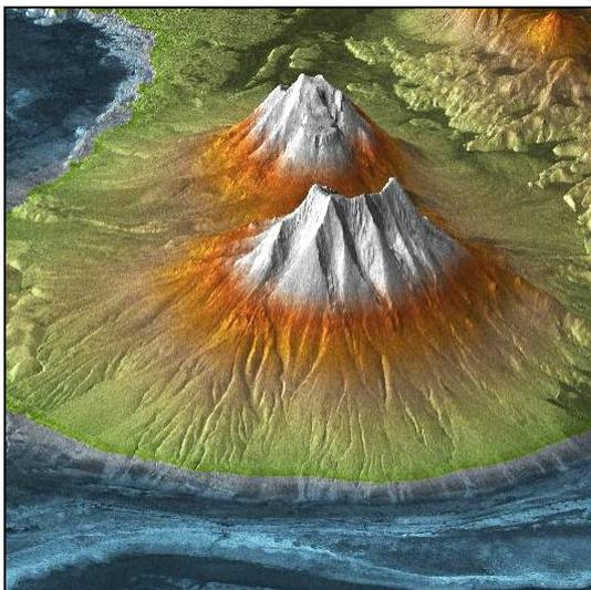
Digital Elevation Model obtained by TanDEM-X of volcano in Bolivia (copyright DLR).
