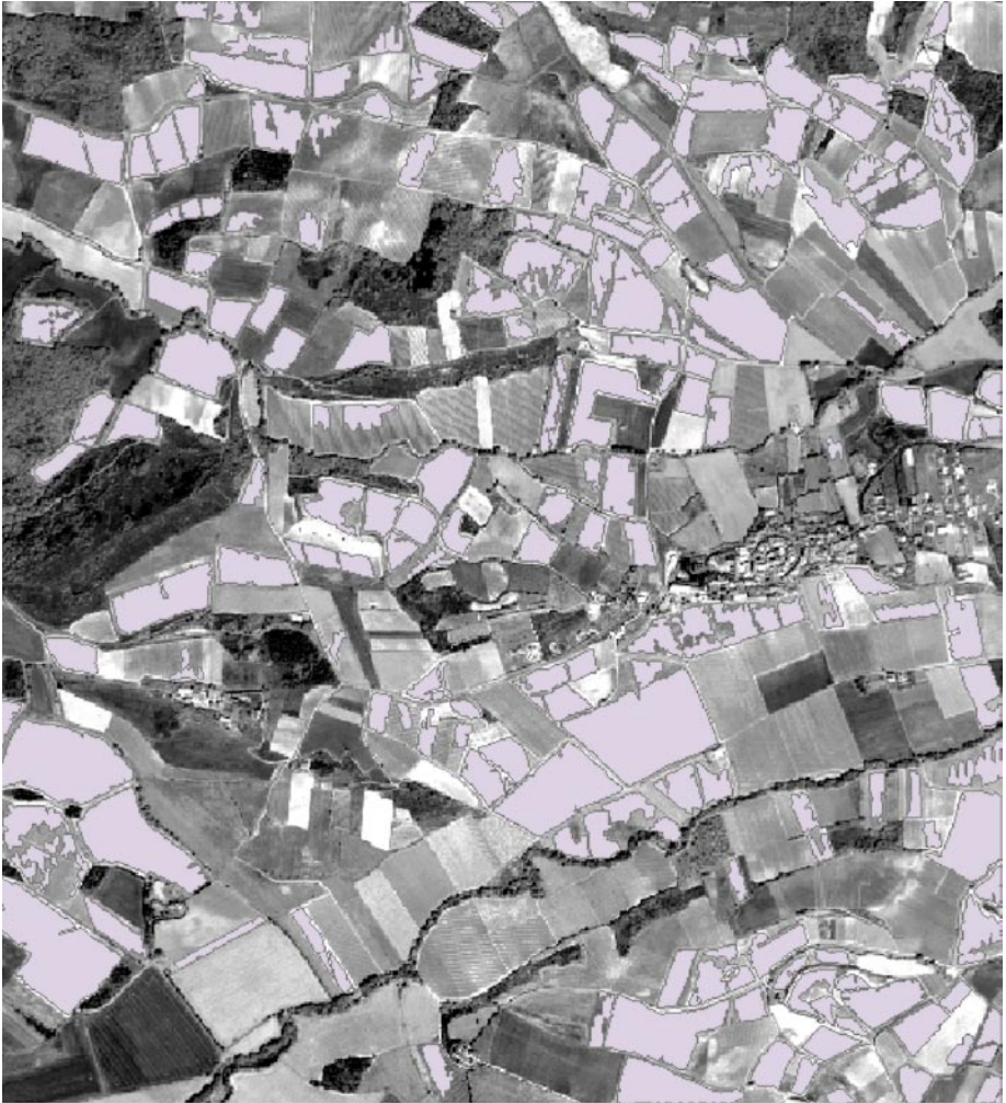
FIGURE.4.16. RESULT OF THE SEGMENTATION ON THE PANCHROMATIC CHANNEL OF THE QUICKBIRD IMAGE, LIMOUX TEST-SITE (FRANCE)
