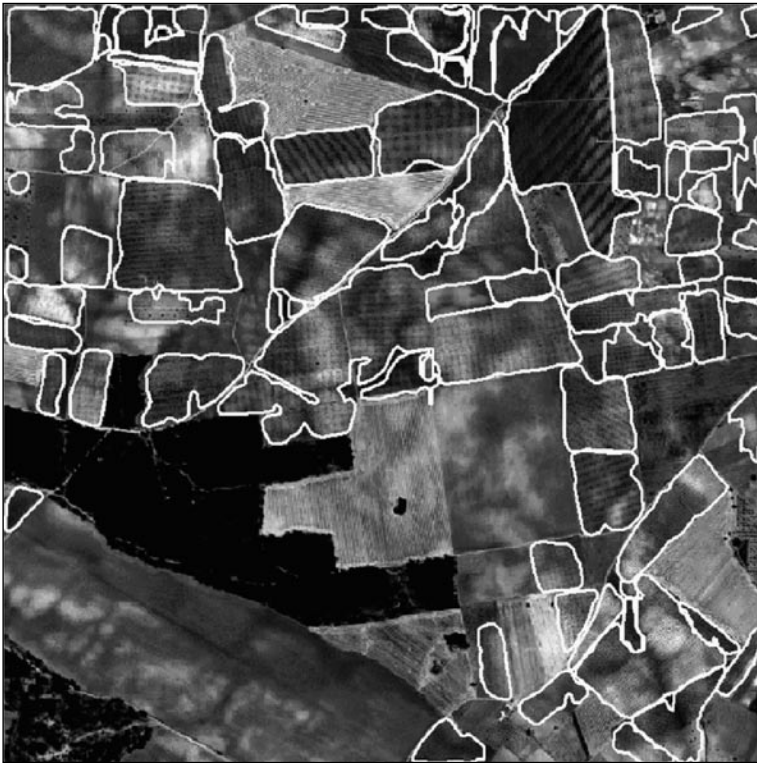
FIGURE 4.17. RESULT OF THE SEGMENTATION ON THE PANCHROMATIC CHANNEL OF THE QUICKBIRD IMAGE, 2500x2500 PIXELS EXTRACT, TARAZONA TEST-SITE (SPAIN)
